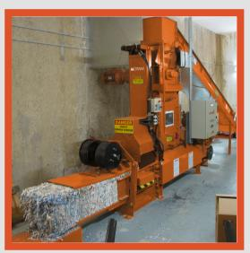
Thanks to the narrow channel, model 2050 AT and 15 AT are ideal for compaction of shredded paper, offcuts and other small pieces of material.
