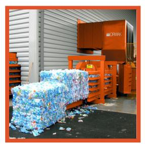
The sturdy large balers in our horizontal range are designed to compact tough material such as empty PET bottles and aluminum cans.
